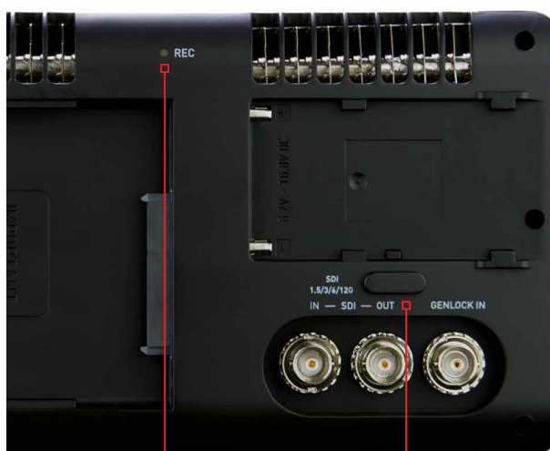
Tally Light Flashes red when recording
